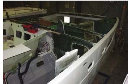
Catana 50 in build – note composite bulkheads everywhere
